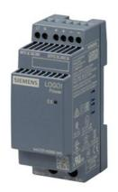
SIPLUS LOGO! Power 24V 1,3A for medial stress -40...+70°C start up at -25°C based on 6EP3331-6SB00-0AY0 . stabilized power supply input: AC 100-240 V output: DC 24 V / 1,3 A
