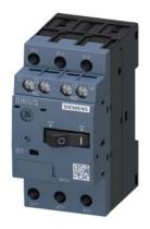
Circuit breaker size S00 for motor protection, CLASS 10 A-release 3.5...5 A N release 65 A 1 NO+1 NC transverse Screw terminal Standard switching capacity
