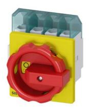
SENTRON, Switch disconnector 3LD, emergency switching-off switch, 4-pole, Iu: 32 A, operating power / at AC-23 A 400 V: 11.5 kW, front-mounted, rotary operating mechanism, Red / yellow, 4-hole mounting of the handle
