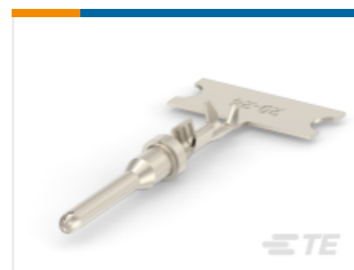
TE Part #3-2600020-2 XRC PIN TERMINAL 14-18AWG Ni Plated
