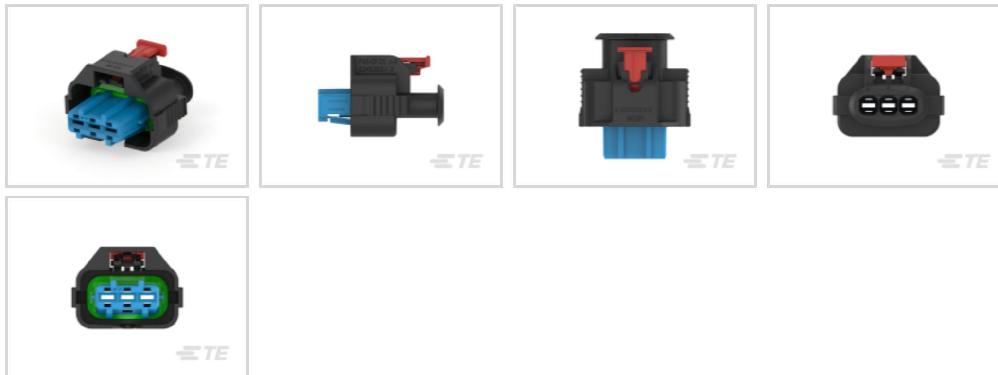
Connector System: **Cable-to-Cable**Number of Positions: **3**Connector & Housing Type: **Receptacle**Sealable: **Yes**Mating Tab Width: **2.8 mm [ .109 in ]**
