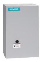
2-speed 3-phase motor starter Size 4 Two separate windings Constant or variable torque Solid-state overload relays Low SPD OLR range 50-200A High SPD OLR range 50-200A 110-120/220-240VAC 60HZ coil Enclosure NEMA type 1 Indoor general purpose use
