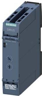
Timing relay, electronic OFF delay without control signal or smooth passing make contact non-volatile 7 time ranges 0.05...600 s 12-240 V AC/DC at 50/60 Hz AC, 1 change-over contact with LED Spring-type terminal (push-in)
