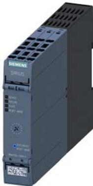
Direct starter, 3RM1, 500 V, 0.09 - 0.75 kW, 0.4 - 2 A, 110-230 V AC, screw/spring-type terminals
