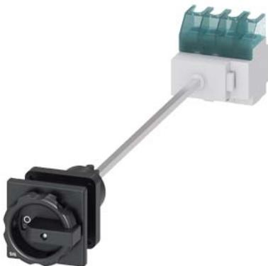
SENTRON, Switch disconnector 3LD, main switch, 4-pole, I<sub>u</sub>: 25 A, Operating power / at AC-23 A at 400 V: 9.5 kW, floor mounting with door coupling, rotary operating mechanism, black, central mounting 22.5 mm of the handle
