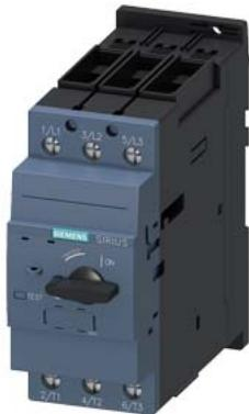
Circuit breaker size S2 for starter combination Rated current 45 A N-release 650 A screw terminal Standard switching capacity
