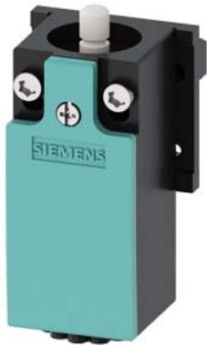
Position switch Plastic enclosure, 31 mm according to EN 50047 Control cabinet type 1 NO/1 NC snap-action contacts integrated (not replaceable) Rounded plunger Degree of protection IP40, with Self-sealing grommet Cover flat, turquoise With accessories: screws and mounting plate without locking sheet metal and seal
