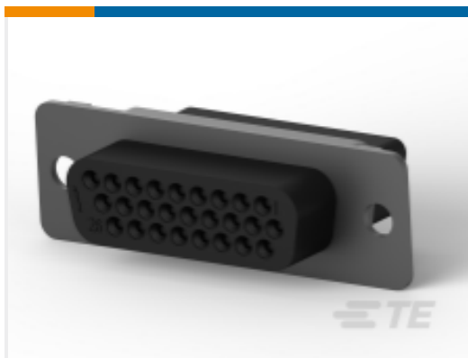
TE Part #1658689-1 D-Sub Crimp Recpt Signal 26 Posn, Socket Size 22, Shell Size 2
