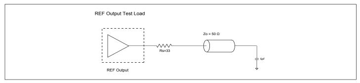
Figure 2. CMOS REF Test Circuit
