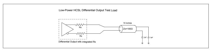
Figure 1. Low Power HCSL Test Circuit
