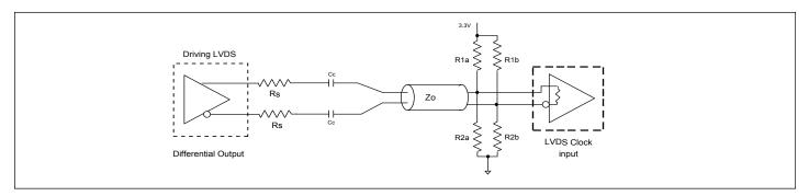
Figure 3. Differential Output driving LVDS
