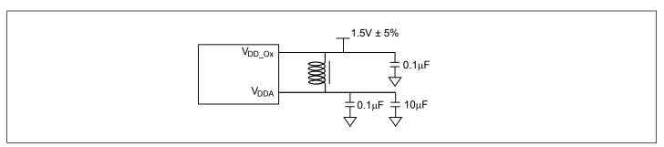
Figure 4. Power Supply Filter
