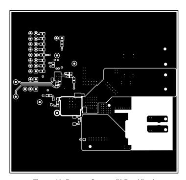
Figure 16. Bottom Copper (X-Ray View)
