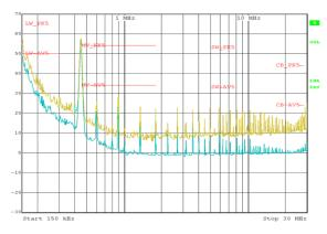
Figure 8. Conducted EMI Test Result 150kHz to 30MHz
