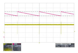
Figure 6. No Load Skip Cycle Operation(C1:Switch Node, C2: V<sub>LOAD</sub>)
