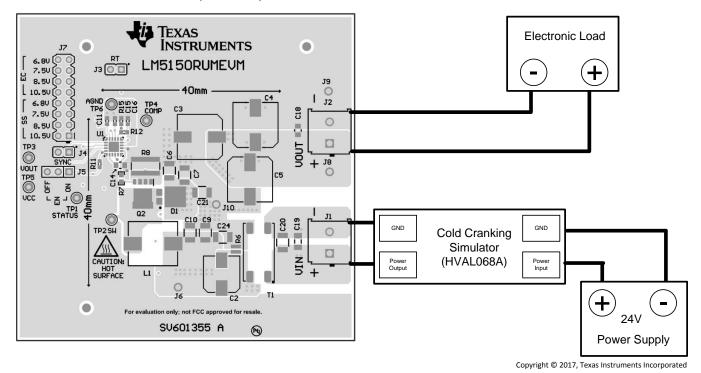
Figure 2. Cranking Simulator Connection Diagram
