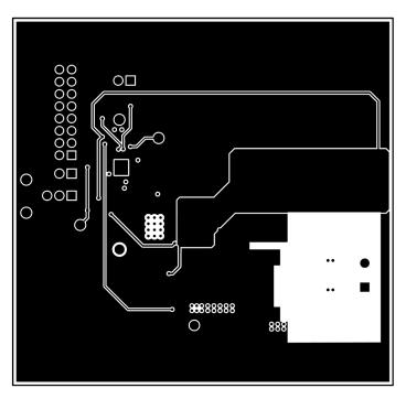
Figure 15. Mid2 Copper (X-Ray View)
