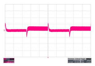
Figure 7. Load Transient(C2:V<sub>LOAD</sub> AC-coupled)
