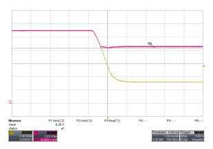
Figure 5. Cold-Cranking Using Cranking Simulator(C1:V<sub>SUPPLY</sub>, C2: V<sub>LOAD</sub>)
