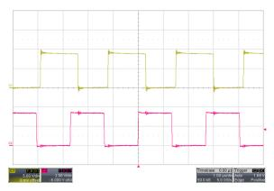
Figure 4. Clock Synchronization(C1:Switch node, C2:SYNC)
