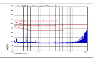
EMI with filter, EN55022 Test method and limits are the same as EN55032.
