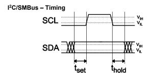
Setup and hold times timing diagram
