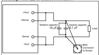
Output ripple and noise test setup
