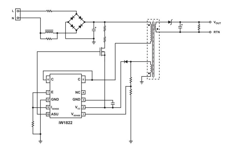
Figure 3.1: iW1822 Typical Application Circuit
