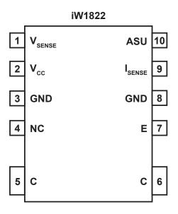
Figure 4.1: 10-Lead SOIC Batwing Package
