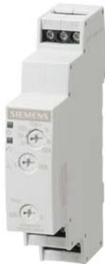
Timing relay, electronic with star-delta (wye-delta) function 2 NO 7 time ranges 0.05 s...100 h 12-240 V AC/DC Screw terminal
