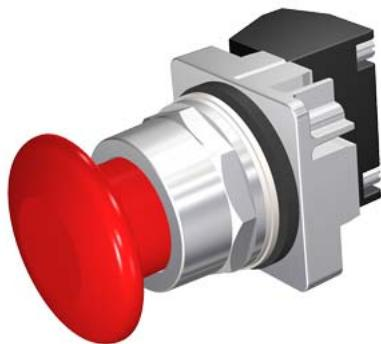
30mm Command/52, Chrome Finish Heavy Duty, Watertight/Oiltight Point-of-Purchase Kit Push-Pull Operator Non-Illuminated Mushroom Head Cap Small 1 3/4" (44.5 mm) Plastic Cap, Red 2 Position Maintained, Pull-to-Release with 1 N.O. - 1 N.C. Heavy Duty Contacts, A600/P600 UL Listed, CSA Certified NEMA 1,3,3R,4,4X,12,13 & Automotive Standards 1 52NL04R (STOP) and 1 52NL04 (STOP) Legend Plate 1 Yellow Backing Plate with Text: EMERGENCY STOP
