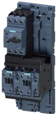
Fuseless motor starter Reversing operation 600VAC Size S0 0.45-0.63A 220/240VAC 50/60HZ screw connection For 35 mm rail-mounting Type of coordination 2 IQ = 150 KA Also full fills type Of coordination 1 1NO+1NC (per contactor)
