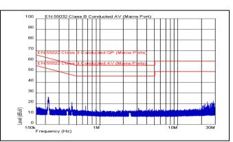
EMI with filter, EN55032. Test method and limits are the same as
