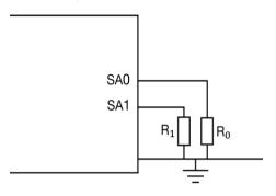
Schematic of connection of address resistors
