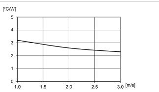
Thermal resistance vs. airspeed measured at the converter. Tested in wind tunnel with airflow and test conditions as per the Thermal consideration  $\label{eq:total_eq} % \begin{center} \end{center} \begin{center} \end{center}$ section.  $V_1 = 54 \text{ V}.$
