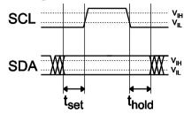
Setup and hold times timing diagram
