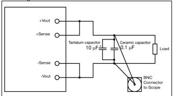
Output ripple and noise test setup
