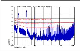
EMI without filter. EN55032 Test method and limits are the same as EN55022. 220 uF 100V input capacitor and 2 x 1 mF 16 V OS-CON output capacitor used.
