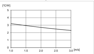
Thermal resistance vs. airspeed measured at the converter. Tested in wind tunnel with airflow and test conditions as per the Thermal consideration section.  $V_1 = 54 \text{ V}.$
