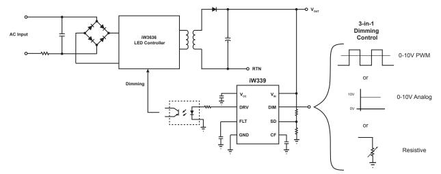
Figure 3.1 : iW339 Typical Application Circuit
