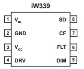
Figure 4.1 : 8-Lead SOIC Package
