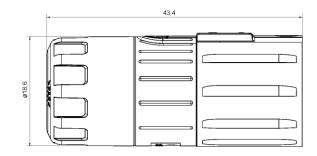
Main Dimensions Plug \*for max. wire cross-section pay attention to the cross-section of used contacts
