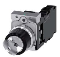
RONIS key-operated switch, 22 mm, round, metal, shiny, lock number SB30, with 2 keys, 2 switch positions O-I, latching, actuating angle 90°, 10:30h/13:30h, key removal O+I, with holder, 1 NO+1 NC, screw terminal, possible special locks: SB31, 421, 455
