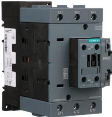
Electrically held lighting contactor, Contactor amp rating 100A, 0 N.C. / 3 N.O. Poles, 110VAC 50HZ/120VAC 60HZ coil, 1 NO / 1 NC auxiliary contacts Non-combination type, (no disconnect device), Enclosure NEMA type (open), No enclosure
