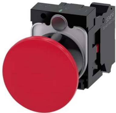
Mushroom pushbutton, 22 mm, round, plastic, red, 40mm, latching, pull-to-unlatch mechanism, with holder, 1 NC, spring-type terminal, with laser labeling, upper case and lower case, always upper case at the beginning of the word
