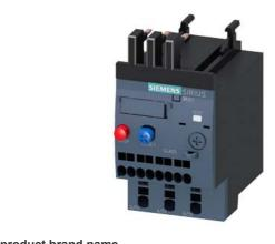
Overload relay 1.8...2.5 A Thermal For motor protection Size S00, Class 10 Contactor mounting Main circuit: Spring-type terminal Auxiliary circuit: spring-type terminal Manual-Automatic-Reset
