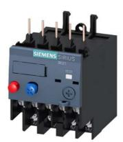
Overload relay 4.5...6.3 A Thermal For motor protection Size S00, Class 10 Contactor mounting Main circuit: Ring cable lug Auxiliary circuit: ring cable lug Manual-Automatic-Reset
