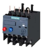
Overload relay 0.45...0.63 A Thermal For motor protection Size S00, Class 10 Contactor mounting Main circuit: Ring cable lug Auxiliary circuit: ring cable lug Manual-Automatic-Reset
