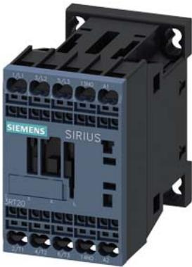
power contactor, AC-3 9 A, 4 kW / 400 V 110 V AC, 50 Hz, 120 V, 60 Hz, 3-pole, Size S00 Spring-type terminal Multi-unit packaging 32 units
