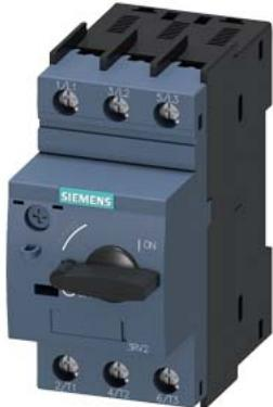
Circuit breaker size S00 for motor protection, CLASS 10 A-release 1.8...2.5 A N-release 33 A screw terminal Standard switching capacity Multi-unit packaging Pack = 24 units
