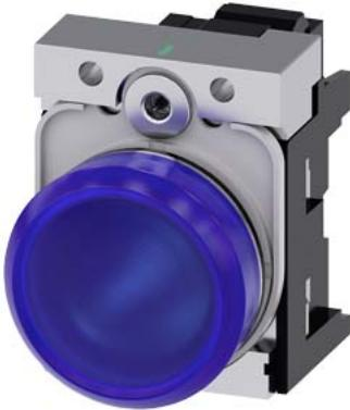
Indicator lights, 22 mm, round, metal, shiny, blue, lens, smooth, with holder, LED module with integrated LED 24 V AC/DC, spring-type terminal, with laser labeling, upper case
