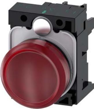
Indicator lights, 22 mm, round, plastic, red, lens, smooth, with holder, LED module, with integrated LED 24 V AC/DC, screw terminal, with laser labeling, inscription or symbol Customer-specific selection with SIRIUS ACT configurator (CIN)
