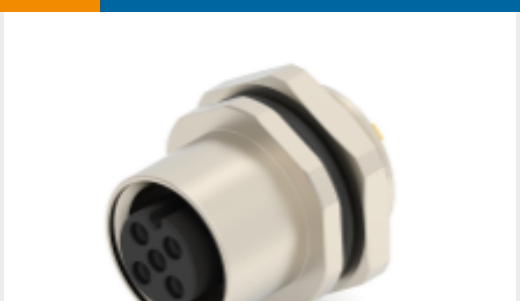
TE Part #T4133012051-000 M12,FRONT MOUNT,FEMALE,A,5P, SOLDER WIRE
