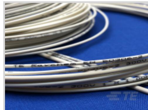
Cable Type: **Primary Wire**Wire & Cable Insulation Material: **Halogen-Free Polymer**Conductor Material: **Tin Plated Copper**Outside Cable Diameter: **1.3 mm [.051 in]**Wire Size: **20 AWG**[All Single Wire, Thin Wall, EN50306-2 \(0\)](#)
