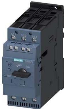
Circuit breaker size S2 for motor protection, CLASS 10 A-release 32...40 A N-release 585 A screw terminal increased switching capacity with transverse auxiliary switches 1 NO+1 NC
