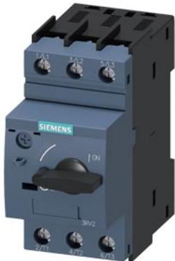
Circuit breaker size S0 for motor protection, CLASS 10 A-release 11...16 A N-release 208 A screw terminal Switching capacity 30 kA at 600 V according to UL/CSA
