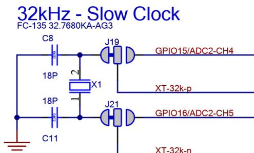
Figure 12: Schematic - 32 kHz crystal
