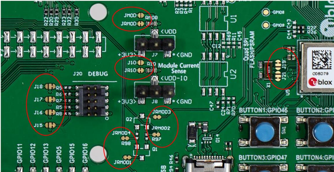
Figure 17: PCB jumper positions – highlighted in red
