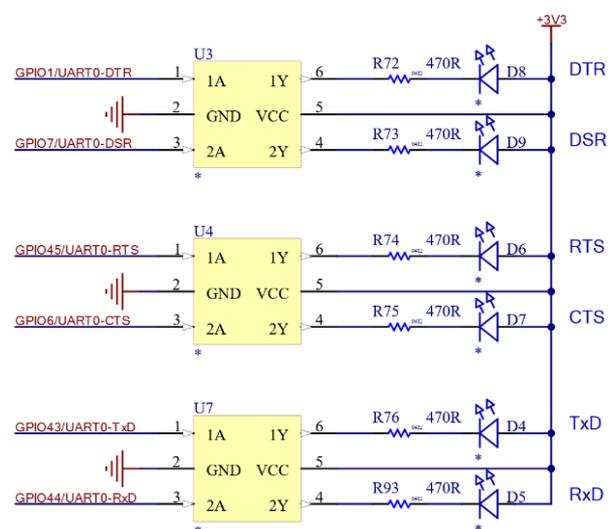
**Figure 9: Schematic – UART0 status LEDs**
