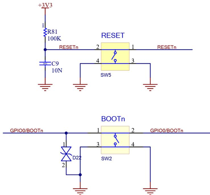
Figure 6: EVK schematic - reset and boot buttons
