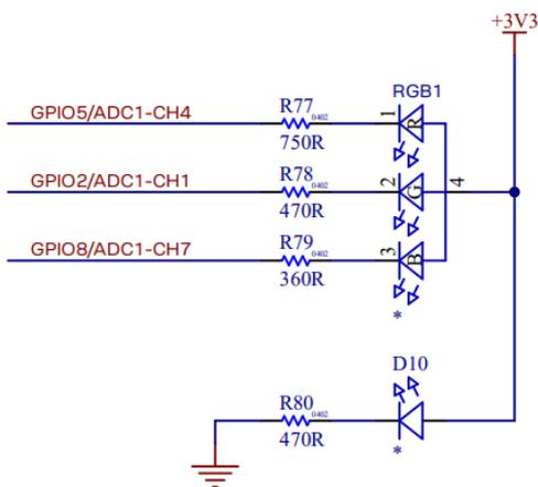
**Figure 8: Schematic – RGB and power LED**
