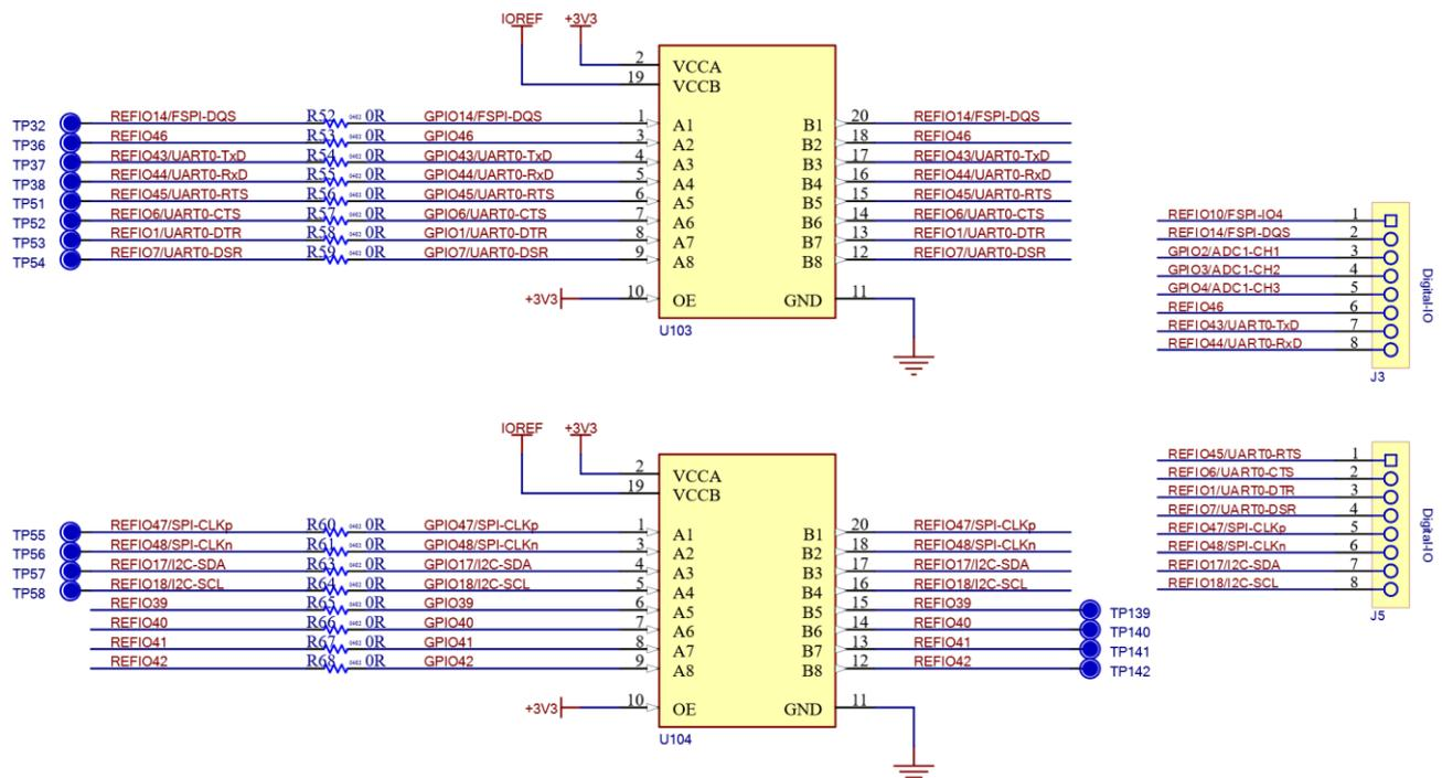
**Figure 10: UART0 level shifters and pin socket**
