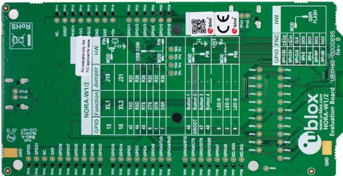
Table 6 shows the default configuration of “solder-bridge” jumpers. Choose alternative configurations by cutting the bridge and soldering the jumpers in the default positions.
