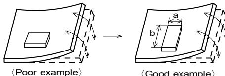
(2) Components location on PCB separation
