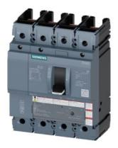
circuit breaker 3VA5 UL frame 250 breaking capacity class M 35kA @ 480 V 4-pole, line protection TM230, FTAM, In=150A overload protection Ir=150A fixed short-circuit protection Ii=5...10 x In N conductor protection 100% without connection
