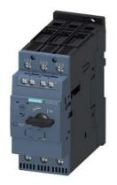
Circuit breaker size S2 for motor protection, CLASS 10 A-release 35...45 A N-release 650 A screw terminal increased switching capacity with transverse auxiliary switches 1 NO+1 NC
