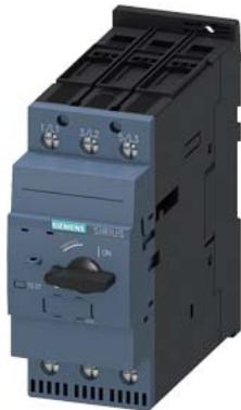
Circuit breaker size S2 for starter combination Rated current 52 A N-release 741 A screw terminal Standard switching capacity
