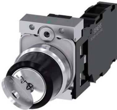
RONIS key-operated switch, 22 mm, round, metal, shiny, lock number SB30, with 2 keys, 2 switch positions O-I, latching, actuating angle 90°, 10:30h/13:30h, key removal O+I, with holder, 1 NO+1 NC, screw terminal, possible special locks: SB31, 421, 455 upper case and lower case, always upper case at the beginning of the word
