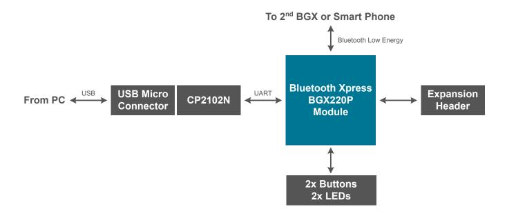
Figure 2.1. BGX220P Expansion Board Block Diagram
