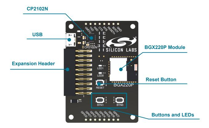
Figure 3.1. BGX220P Expansion Board Hardware Layout
