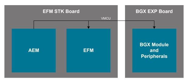
Figure 7.2. Measuring BGX220P Expansion Board Current Using AEM
