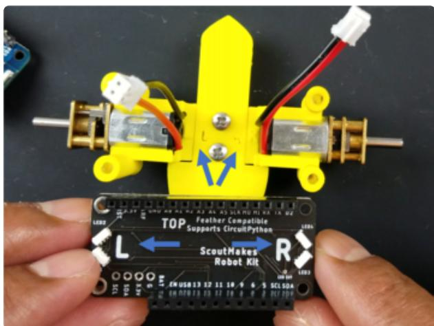
Connect the motor wires to the robot board. Notice the orientation of the robot board with the TOP facing up. Ensure the R to R and L to L are lined up with the robot chassis and robot board.
