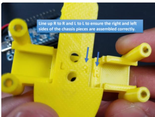
Assemble the robot chassis by bringing together the 2 plastic pieces. Ensure the sides line up as in the image below.
