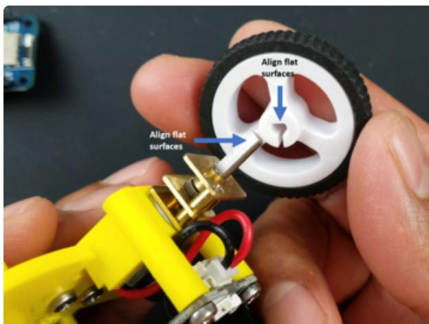
Install the wheels onto the motors. The wheels just press-fit onto the motor shaft. Ensure the flat surfaces on the motor and wheel line up and press.
