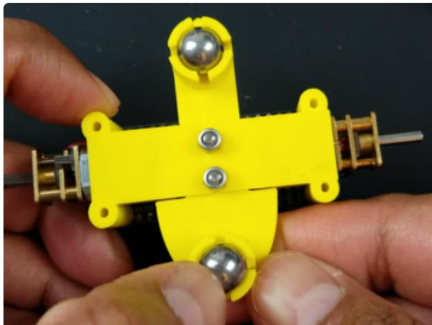
Press fit the 2 ball bearings onto the caster holders.
