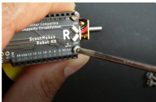
Screw in the robot board to the chassis using the 4 short screws provided. Ensure that the L and R orientation of the board is correct prior to screwing in.
