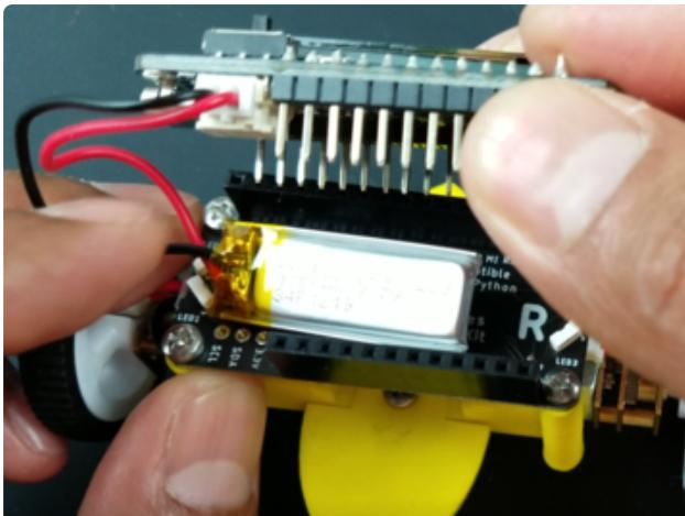
Connect the Azul bluetooth board to the robot board. Ensure the headers line up correctly prior press fitting the 2 boards. The lithium polymer battery can be tucked between the 2 boards.
