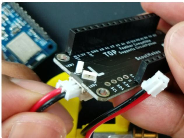
Push in the motor connectors to the board. They can only be inserted in one direction, so don't worry about reversing the connection.
