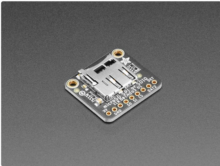
Micro SD cards and microcontrollers go together like micro-peanutbutter-and-jelly: SD cards are inexpensive, durable, easy to find at any shop, come in many sizes and can plug into any computer using a common SD card reader. That makes them perfect for microcontroller storage and retrieval - whether it's images, fonts, GIFs, audio files, or sensor logs.
