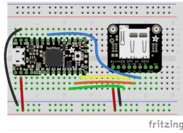
Board 3V to breakout 3V via supply rail
