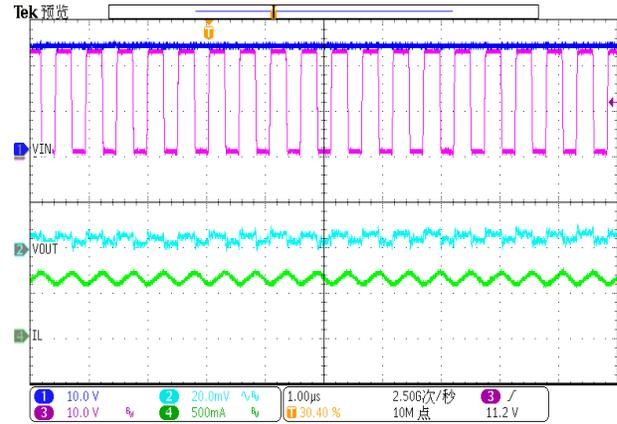
Figure 21. SW and Vout Ripple ( $I_{out}=0.6A$ )
