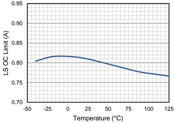
Figure 7. LS Current Limit VS Temperature
