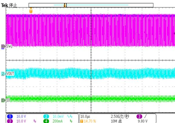
Figure 22. SW and Vout Ripple ( $I_{out}=0A$ )
