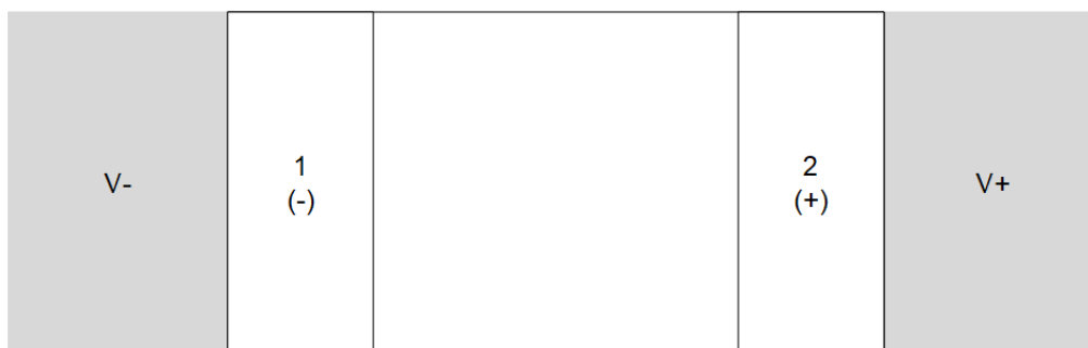
Figure 10-1. DEC Package Recommended Layout
