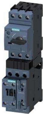
FUSELESS LOAD FEEDER DIRECT START, AC 400V, SZ. S0, 7...10A, AC 110/120V 50/60HZ SCREW TERMINAL FOR RAIL MOUNTING, TYPE OF ASSIGNMENT 2, IQ = 150KA (ALSO FULFILLS TYPE OF ASSIGNMENT 1) 1NO+1NC (CONTACTOR)
