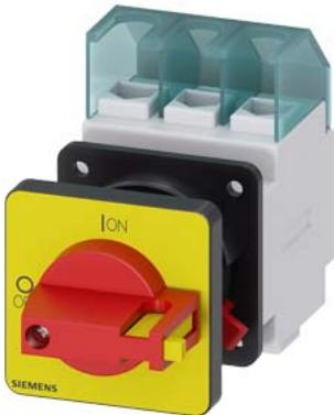
SENTRON, Switch disconnector 3LD, emergency switching-off switch, 3-pole,  $I_{lu}$ : 32 A, operating power / at AC-23 A 400 V: 11.5 kW, front-mounted, knob-operated mechanism, Red / yellow, central mounting 22.5 mm of the handle
