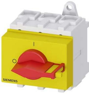
SENTRON, Switch disconnector 3LD, emergency switching-off switch, 3-pole,  $I_u$ : 63 A, operating power / at AC-23 A 400 V: 22 kW, installation in distribution boards, knob-operated mechanism, Red / yellow, handle direct at the switch
